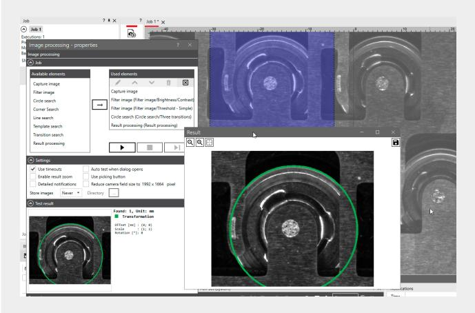
A **result handler** combines the results of the individual searches to calculate offset and rotation for the transformation.
