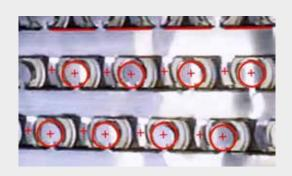
With RAYGUIDE MATCH, features such as edges and circles can be detected on the workpiece and the position of the laser processing is automatically adjusted.
