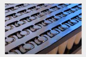
Busbars connect the individual battery cells to form a module with the desired voltage and storage capacity. (Source:Laserax)
