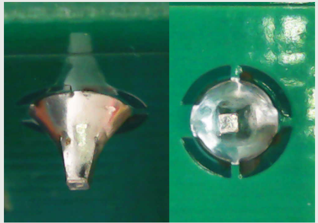
PCB soldering THT example
