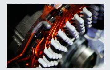
In the hairpin technique, a compressed air gun shoots preformed rectangles of copper wire (similar to hairpins) into slots on the edge of the motor. For each stator, between 160 and 220 hairpins have to be processed within no more than 60 to 120 seconds. After this, the wires are intertwined and welded. Extreme precision is required to preserve the electrical conductivity of the hairpins.
