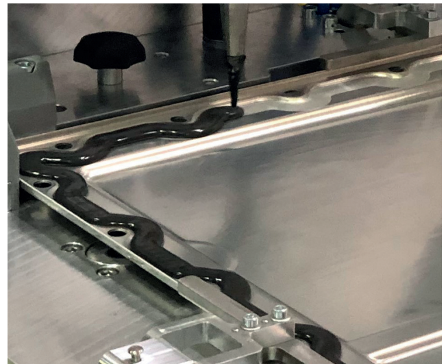
During application of the 1K foam, the robot follows the roughened straight and curved lines created by the laser. Source Robot-Technology
