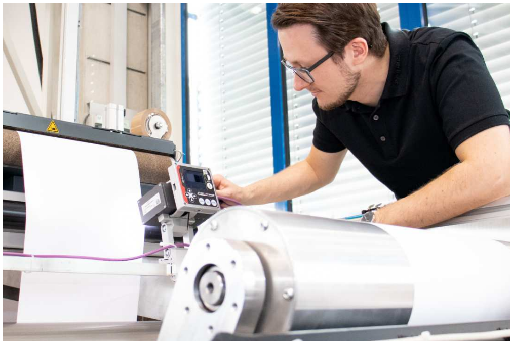
Sonplas Software Engineer Manuel Streifeneder at the roll-to-roll demonstrator: this process is used for cutting electrode sheets. The electrode foils are unwound, cut with the laser and rewound or stacked individually.
