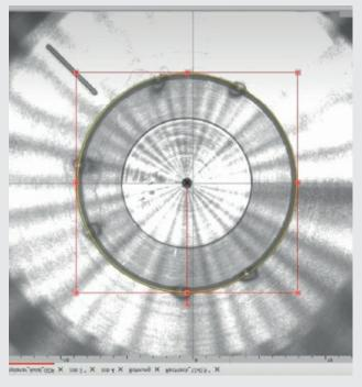
With MACHINE VISION CONTROL (MVC), the laser jobs can be adapted and positioned directly on the component. The MVC is also ideal for automated quality inspection.
