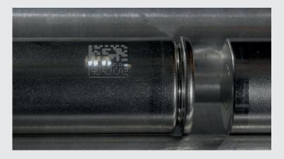
Marking and engraving on 3D surfaces. The dynamic z-axis of the FOCUSSHIFTER RD-14 enables optimum focusing during the marking process. As a result, QR codes and markings remain clearly readable even on uneven surfaces. (Source: Laserax)
