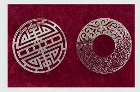
Laser processing of glass. Thanks to the contactfree material ablation, even fragile materials can be processed with the laser. The adjustment of the focus position in the z-direction enables optimum focusing even with thicker glass and thus ensures a precise drilling or cutting result.
