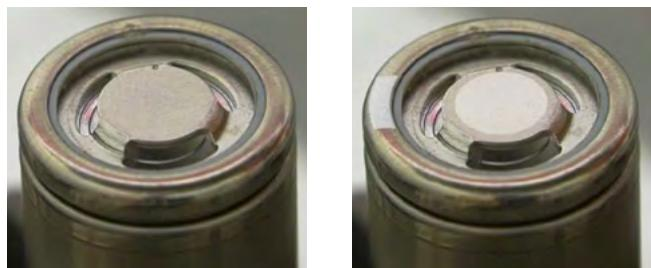
*The top of a cylindrical cell, on the left completely contaminated with oxide and on the right after laser cleaning. Source Laserax*
