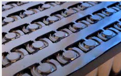
Battery module made of cells connected with laser-welded busbars (source: Laserax)
