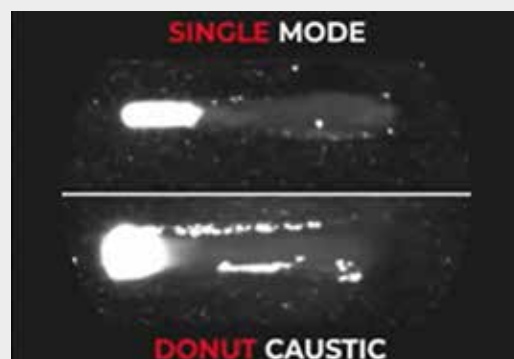
Highspeed camera images of a melting pool with donut and gaussian beam caustics
