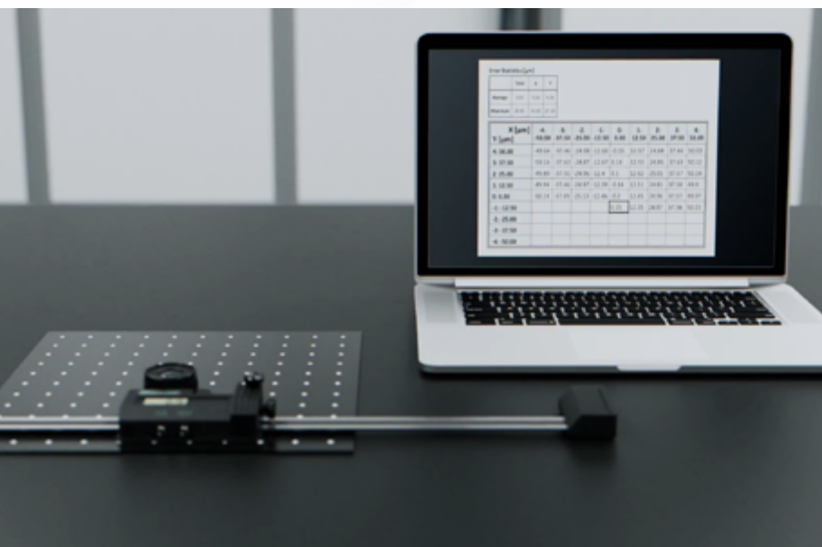
◀ Figure 1: Manual measurement of calibration plates. For the manual calibration of an AM machine, markings are inscribed on a plate in the scan field and then measured. The read values are then transferred to the editor and the deviations are determined and corrected.
