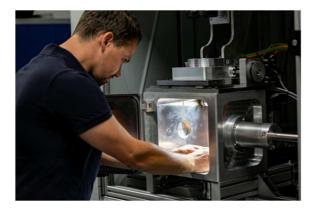
Caption: An employee of LaVa-X works on a laser welding machine with the open evacuation chamber inside. It creates a vacuum over the component in 3 to 5 seconds. Source: LaVa-X
