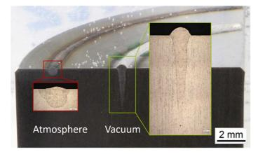
The figure clearly demonstrates the difference between welding in atmospheric conditions and welding under vacuum conditions. The quality of the weld seam is significantly better
