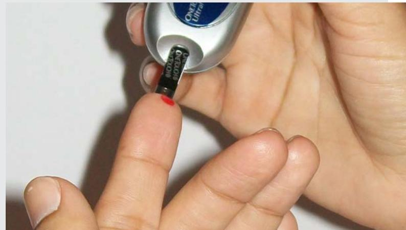
Figure 7: The delicate capillary channels of the blood glucose test strip serve to transport the blood to the sensor
