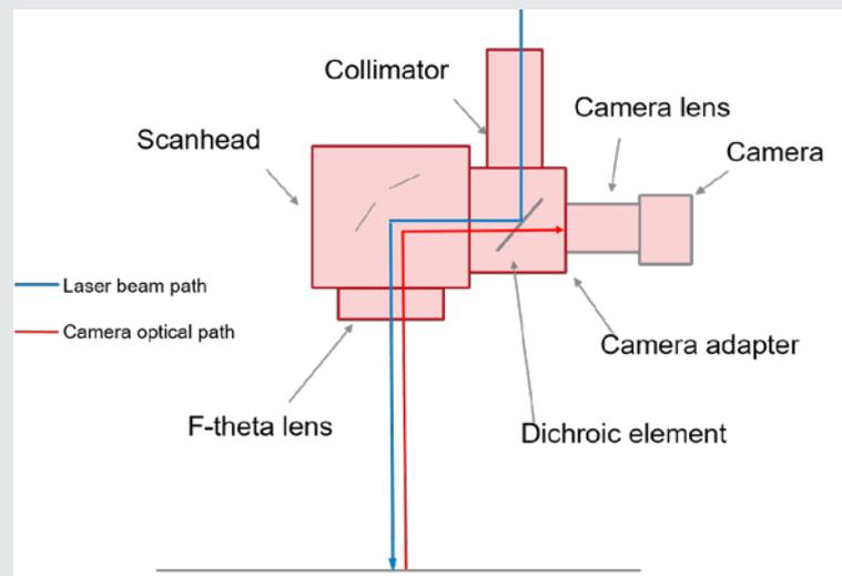
Figure 2: Schematic structure of on-axis machine vision control
