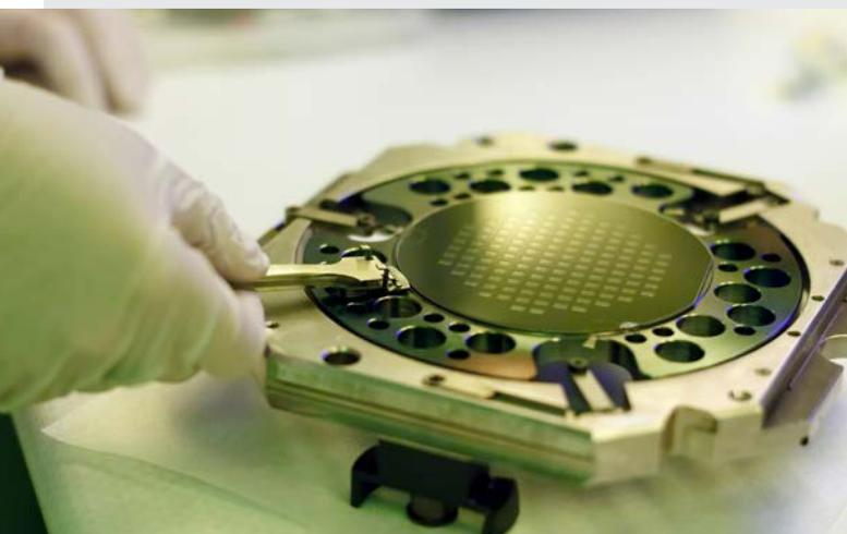
Figure 4: Elaborate holding device for the handling of semiconductor wafers
