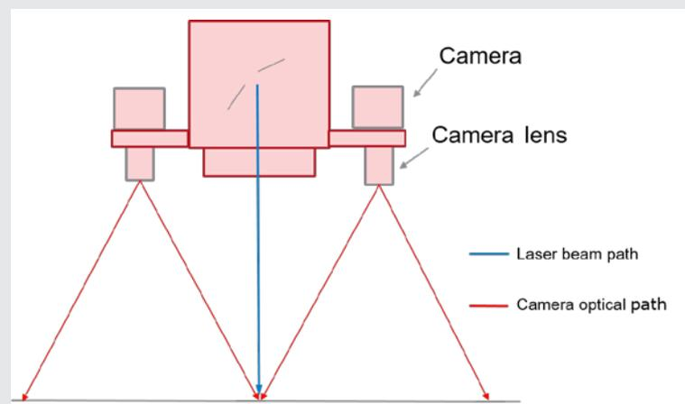
Figure 3: Schematic structure of off-axis machine vision control
