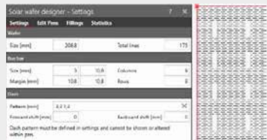
The software solution RAYGUIDE can import or design the customer’s own individual pattern for wafers.
