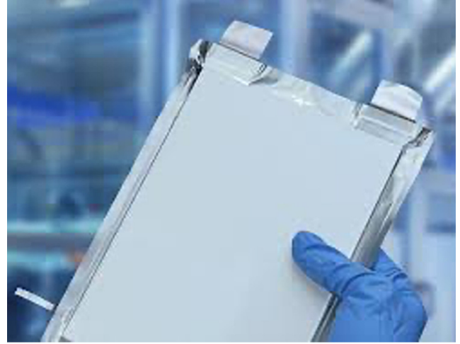
A pouch cell. The "tabs" are clearly visible as contact flags. Source: Fraunhofer Battery Alliance
