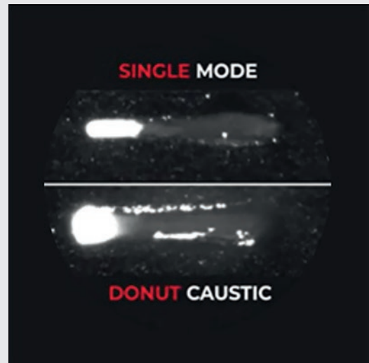
Highspeed camera images of a melting pool with donut and Gaussian caustics
